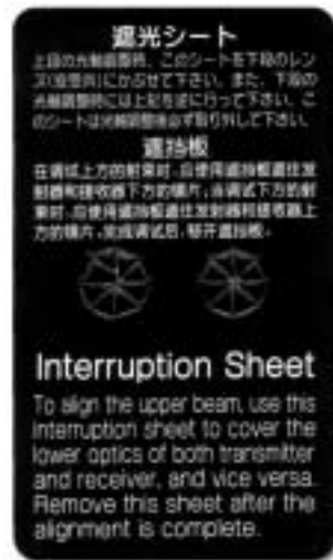
Figure 16: Alignment Interruption Sheet
